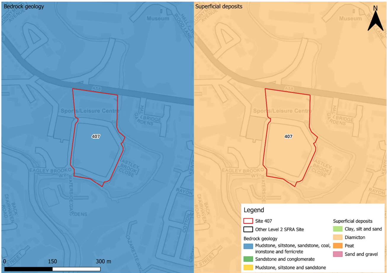
Figure 4-2: BGS Geology - Bedrock and superficial deposits
