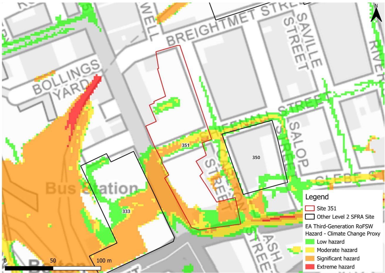
Figure 3-6: 0.1% AEP event surface water flood hazard 1 , as a proxy for the 1% AEP event plus climate change (Third generation - Risk of Flooding from Surface Water map)
