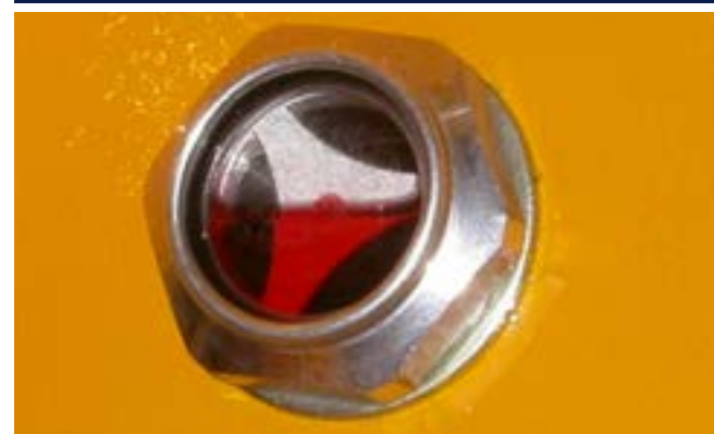
Correct Oil Level when in Centre of Sight Gauge
