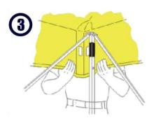
4. Now that the frame is fully expanded, push the sliding leg brackets upwards until ring pull pin locks into position on each leg.
