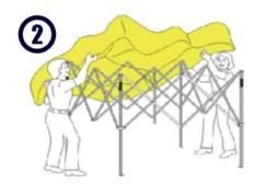
3. Attach velcro securely at each corner. Continue to expand frame completely out.
